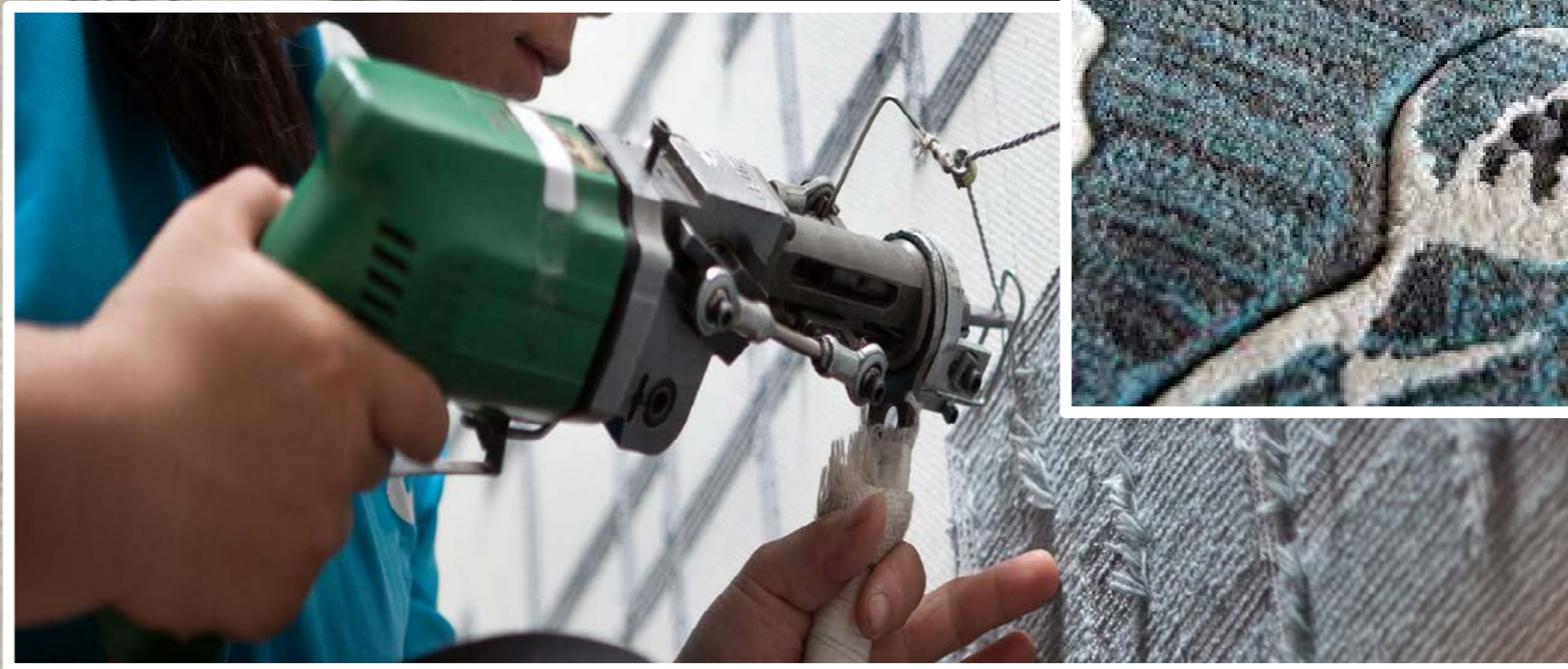
Step 2: Gun Tuft NZ Wool in Loop or Cut into Drawn Design on Backing stretched on Frame from the Back
